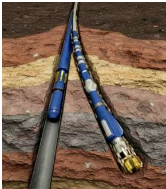
Figure 1: Image of the type of whipstock to be used at the Mt Fuel Skyline Geyser Well.
