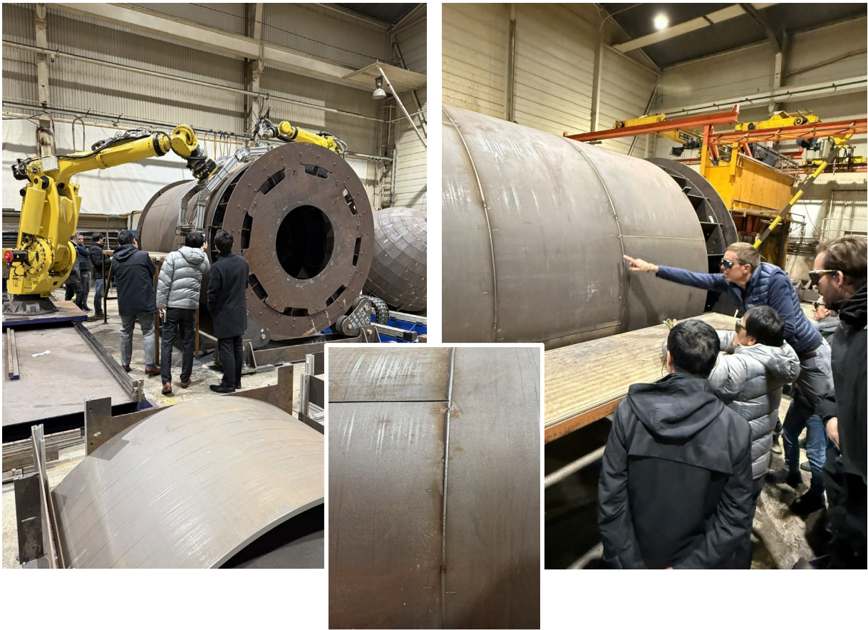
Robotic Cell: Plate handling, mounting, tack welding and seem welds
