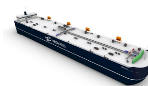
H2Leo barge storage for loading and discharge sites Received AIP from Class (300-600 t H2)
