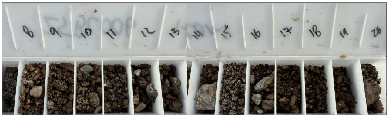
Figure 2: Quartz-goethite alteration in slate host-rock. 25BC006, 6m to 20m.
