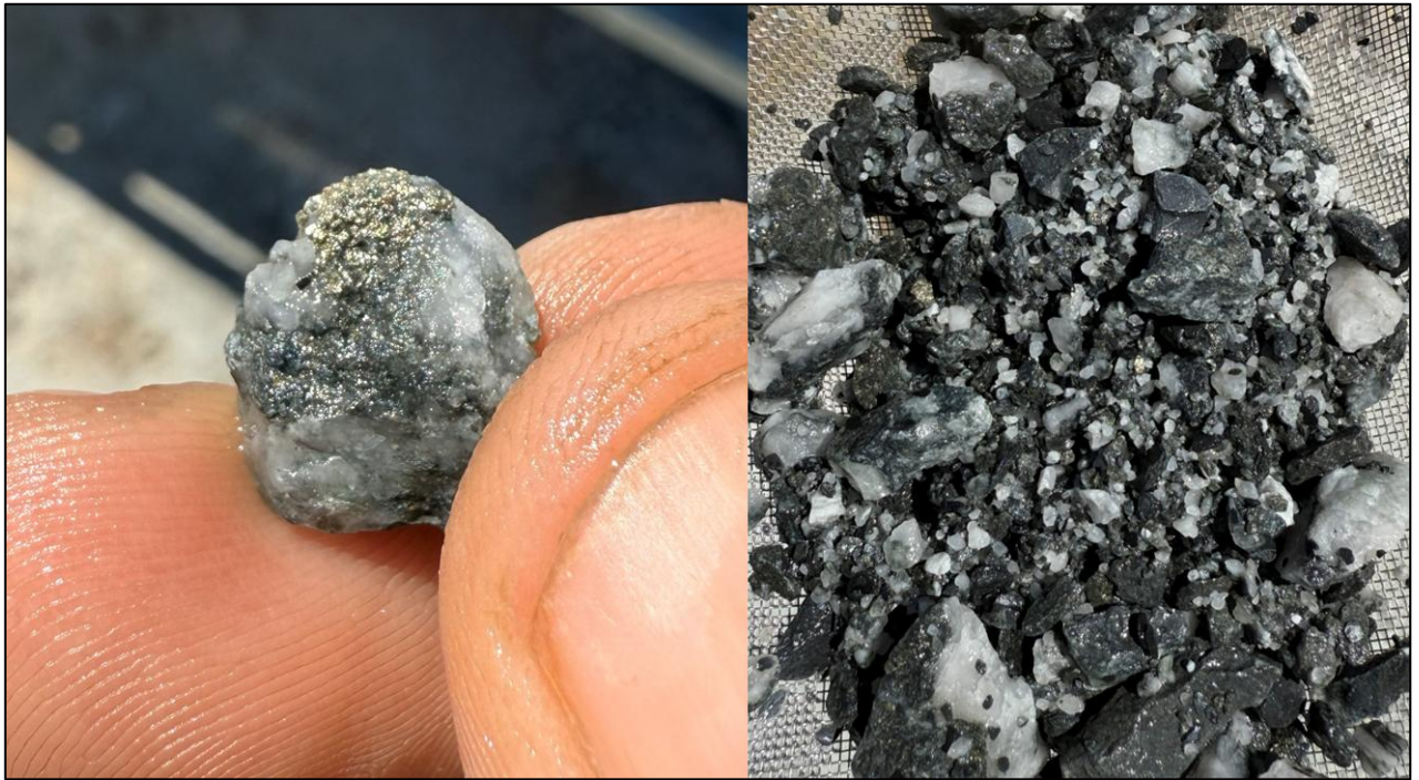
Figure 3: Quartz-pyrite-chlorite alteration in slate host-rock. 25BC002, 179m to 180m.
