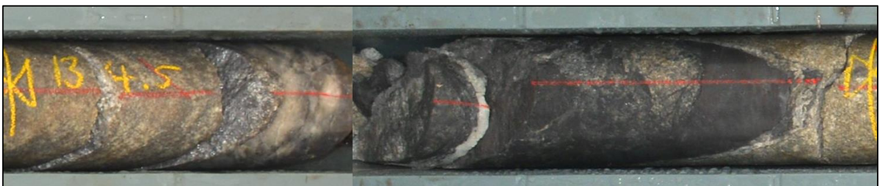
Figure 1: Stibnite and quartz veining from 134.5 to 134.8 which returned 7.33 g/t Au and 4.4% Sb. These zones consistently sit within a broader gold zone and is indicated with moderate to strong sericite alteration.
