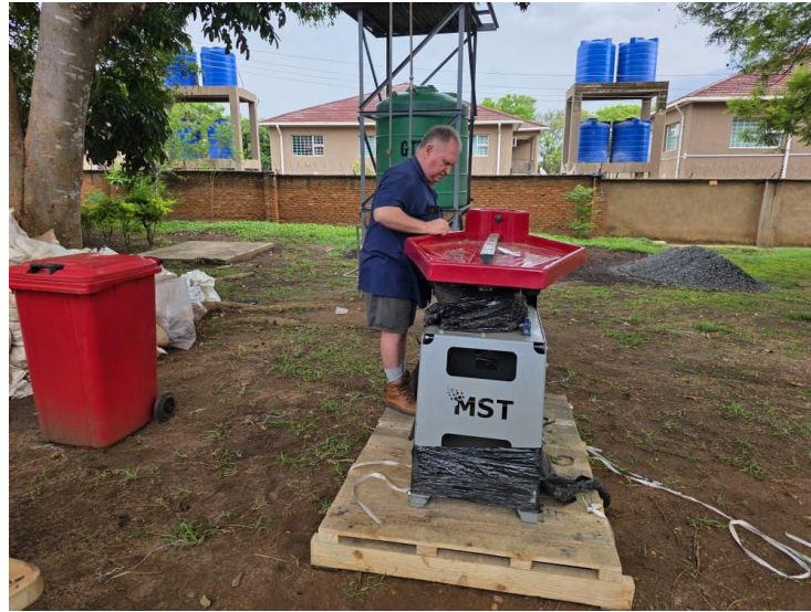
Figure 4. Senior Geologist Leon de Waal inspecting one of the two new Gemini wet shaking tables used for gravity separation during sample processing.
