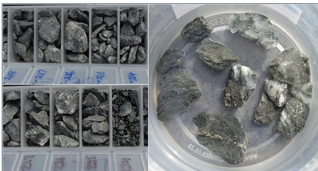
Figure 4: Silicified chips containing quartz veins and pyrite from DRC9. Top left 214-218m, bottom left 224-228m. A selection of chips from DRC9 are shown on the right. Similar chips were seen in DRC10 from 192 to 217m.
