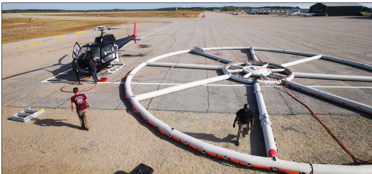
Figure 3: Configuration of Xcite™ TDEM survey system.
