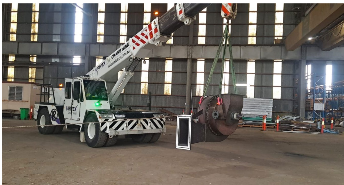
Impellor pre & post coating, dynamic balancing and completed gas transport fan assembly ready for installation and commissioning.
