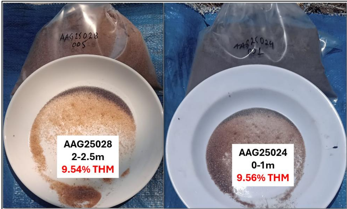
Figure 3: Panned Heavy Mineral Concentrate (HMC) samples from drill samples within Adriano, showing the two highest analytical results THM% from the 37 auger holes drilled Hole AAG15024 is from Area 2 and AAG15028 from Area 4.
