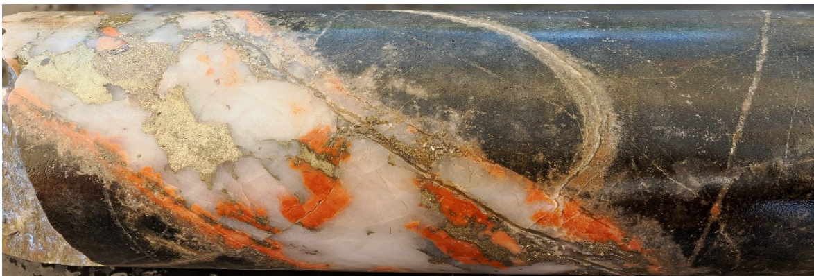
Figure 6. Coarse grained chalcopyrite (yellow) and pyrite (bronze colour) in quartz-feldspar vein cutting volcaniclastic sediments at 378.4m down-hole depth in 25BRD0038. From within a 14m wide interval visually estimated to contain 0.75% chalcopyrite (0.25% Cu*). Core diameter 50mm.
