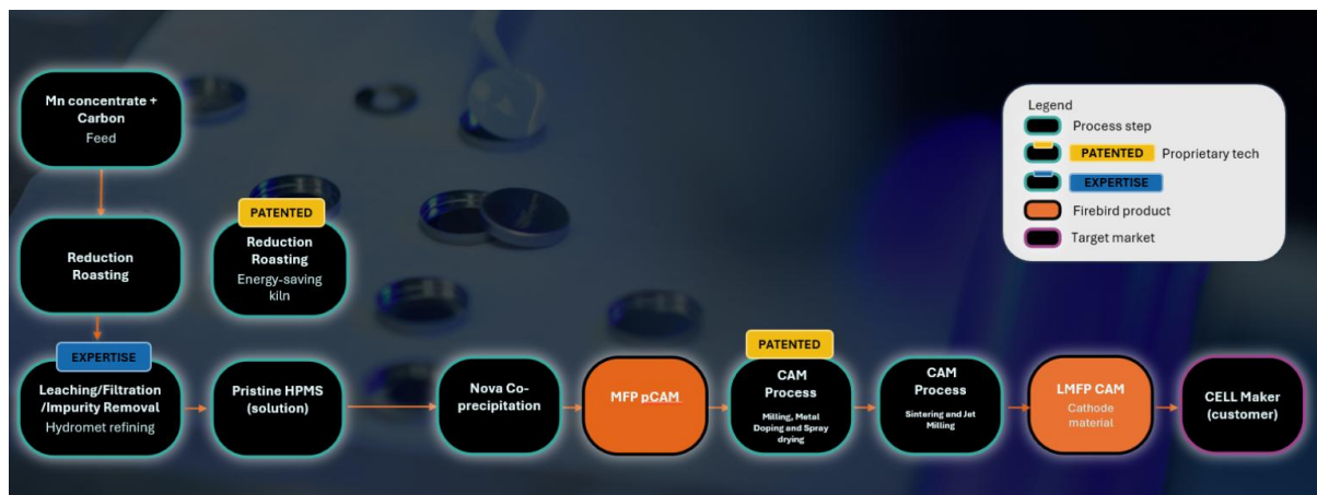
Figure 3. The ADP production process pathway showing the production of MFP PCAM and CAM.
