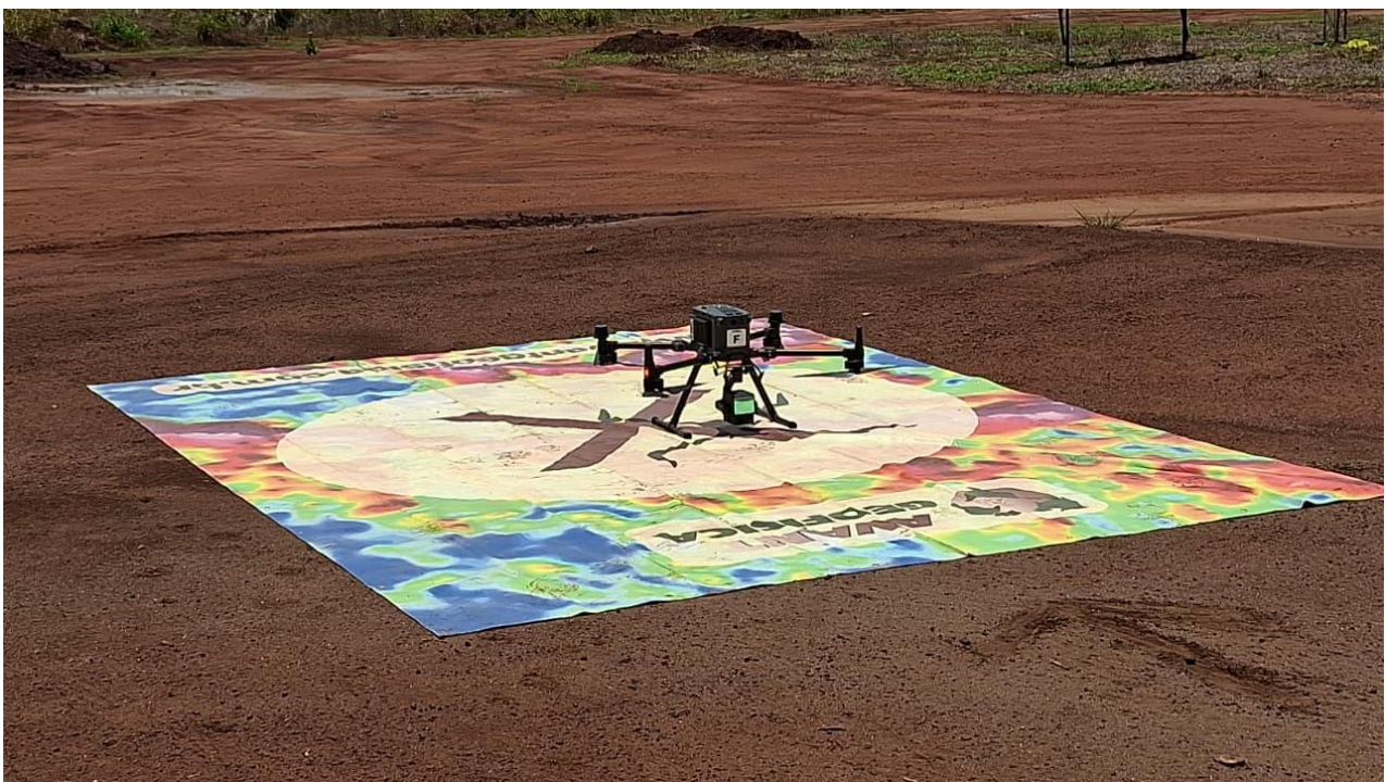
Figure 2: LiDAR sensor mounted below drone while on landing pad at Santa Anna
