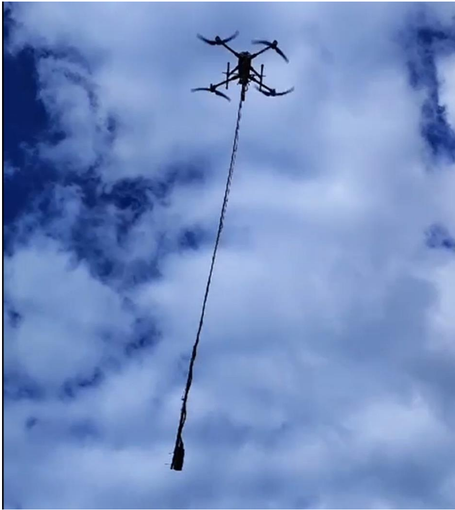
Figure 1: Magnetometer sensor below the drone at Santa Anna
