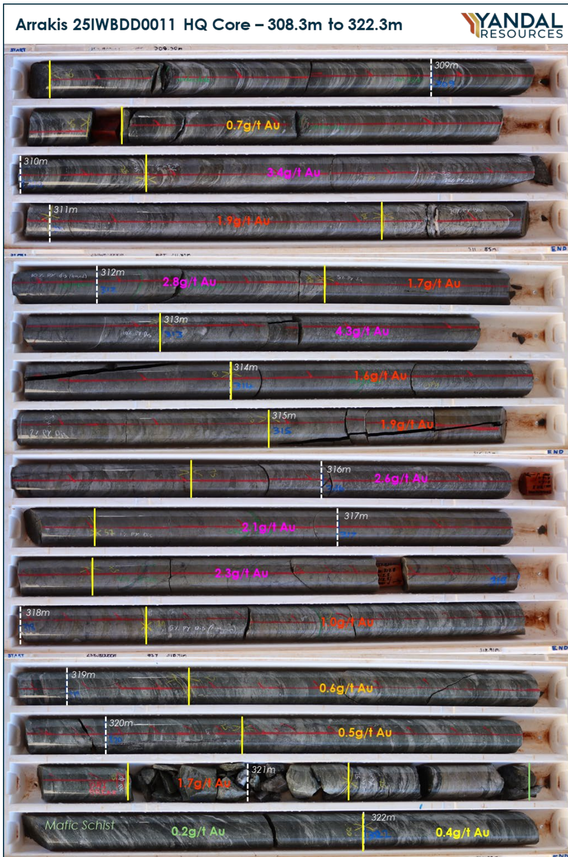
Figure 3: HQ diamond core from 25IWBD0011 showing the mineralisation intercepted that includes 7.95m @ 2.5g/t Au from 310.25m. Metre marks are shown and annotated in white; sample boundaries are marked in yellow.
