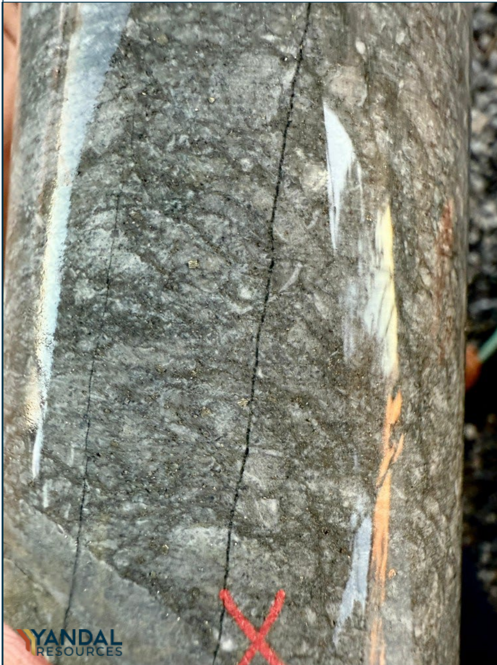
Figure 4: Close up of mineralisation from 25IWBDD0011 from 313.3m to 313.4m, with the broader interval grading at 4.3g/t Au. HQ core has an approximate diameter of 63.5mm.
