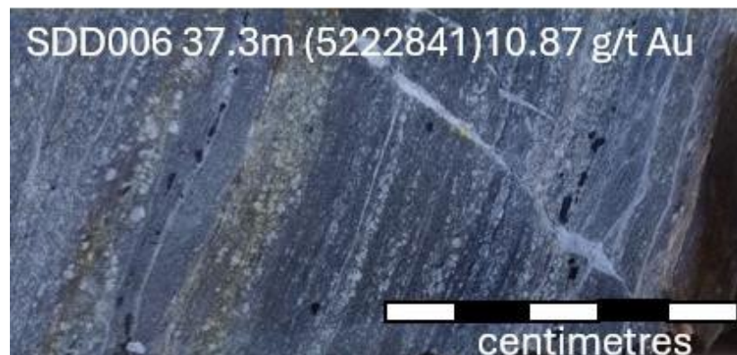
Figure 7. Quartz chlorite schist, chlorite alteration, with trace pyrite-arsenopyrite and a late cross-cutting quartz-carbonate vein. Refer to ASX announcement dated 5 November 2020 for additional information on SDD006 exploration results.
