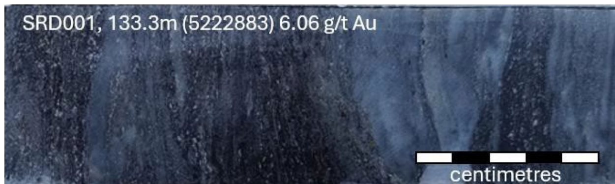
Figure 8. Strong silica-biotite-pyrite alteration, minor chlorite within a dolerite unit. Refer to ASX announcement dated 5 November 2020 for additional information on SRD001 exploration results.
