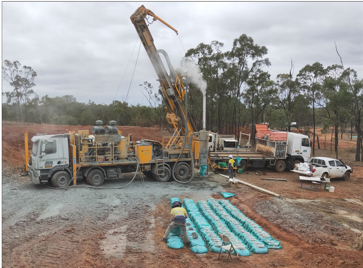
Figure 9. Reverse Circulation drilling and sampling at the Steam Engine Lode
