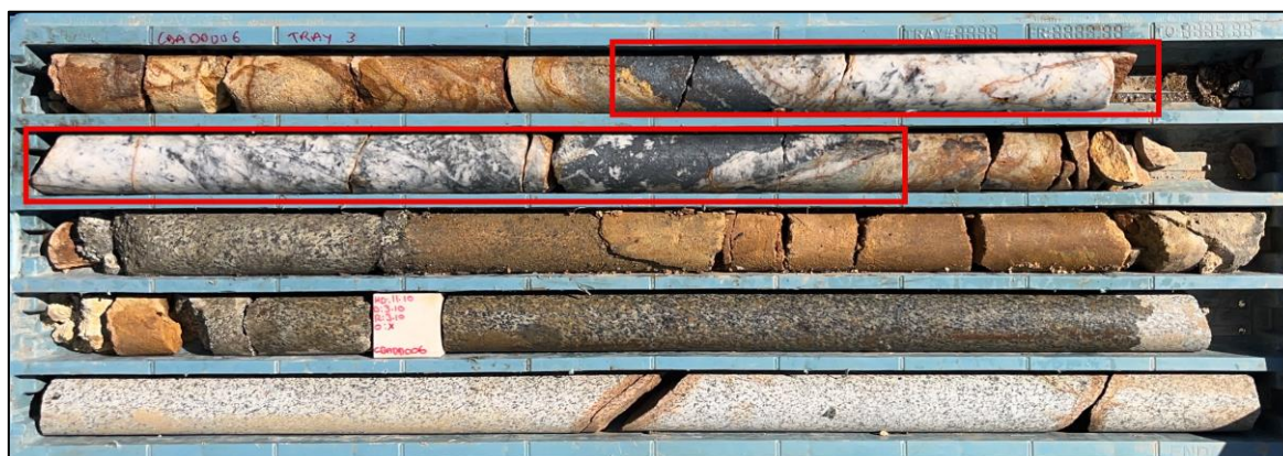
Figure 5 : Section of quartz veining hosting stibnite in hole CBADD006. Interval indicated is from 8.7 to 9.8m and contains massive stibnite from 8.7 to 8.8m, and 9.6 to 9.7m.
