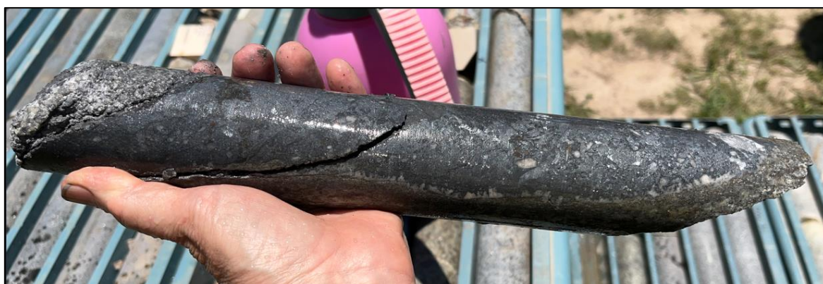
Figure 6: 0.3m of quartz hosted massive stibnite* in hole CBADD007 from 139m. Fault gouge seen on the left of hand specimen, indicating the fault controlled nature of mineralisation at Coonambula.*
