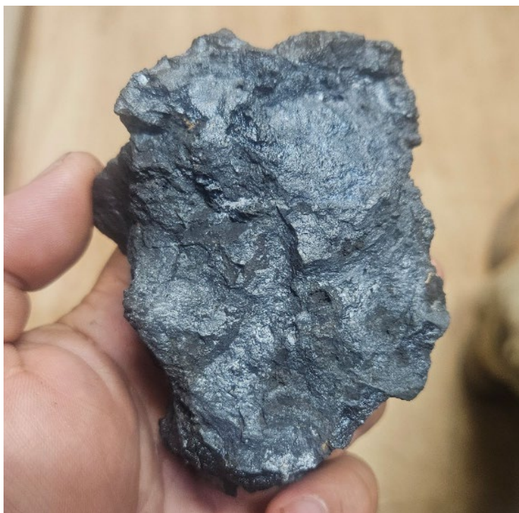
Figure 7: High-grade manganese rock chip sample example with 58.37% Mn (sample ID TKMCCR2506) interpreted to represent near endmember pyrolusite, a high-grade manganese oxide.
