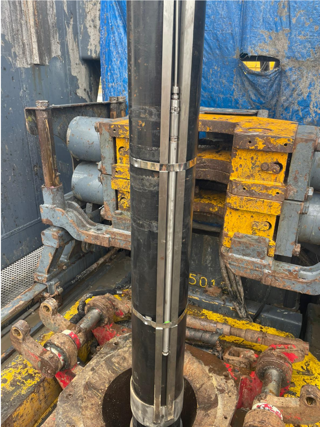
Image 3: Running production casing in Ramsay 3. Note the fiber optic cable attached to the outside of the casing for data collection.
