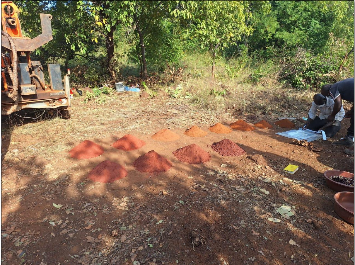
Figure 3: Power auger sampling in progress at Tougbe.
