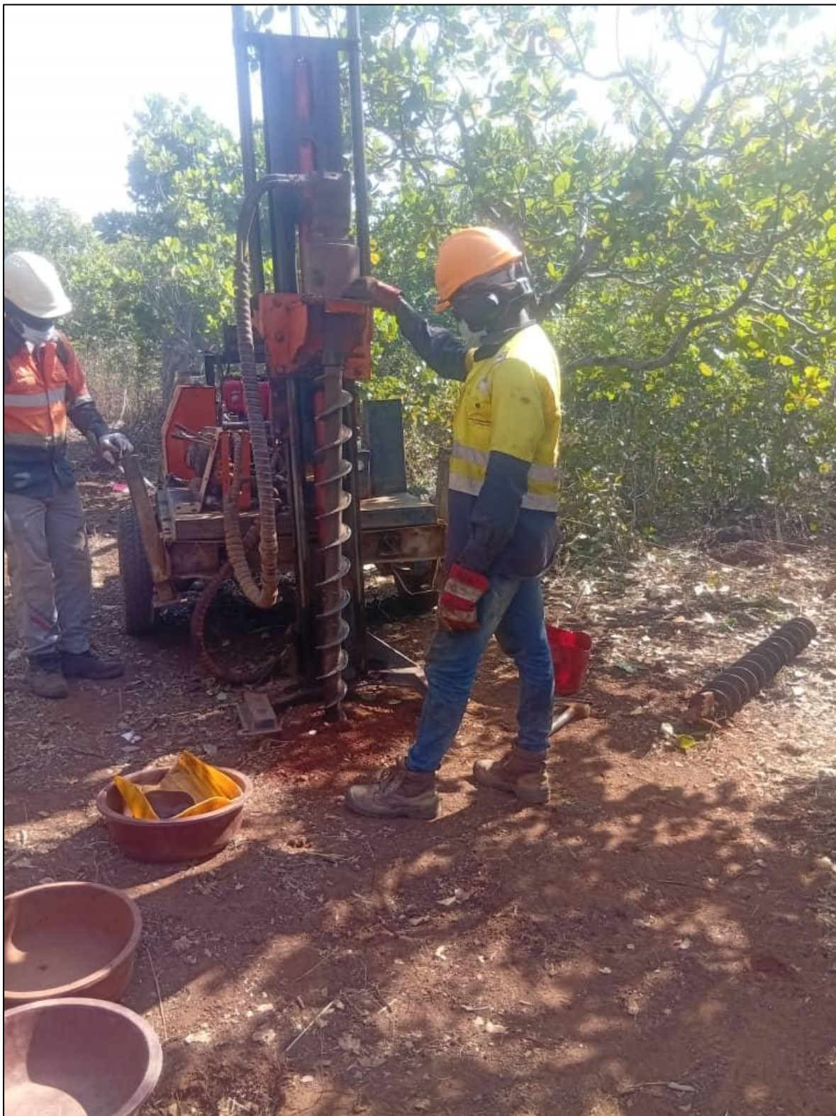
Figure 2: Power auger drilling at Tougbe.
