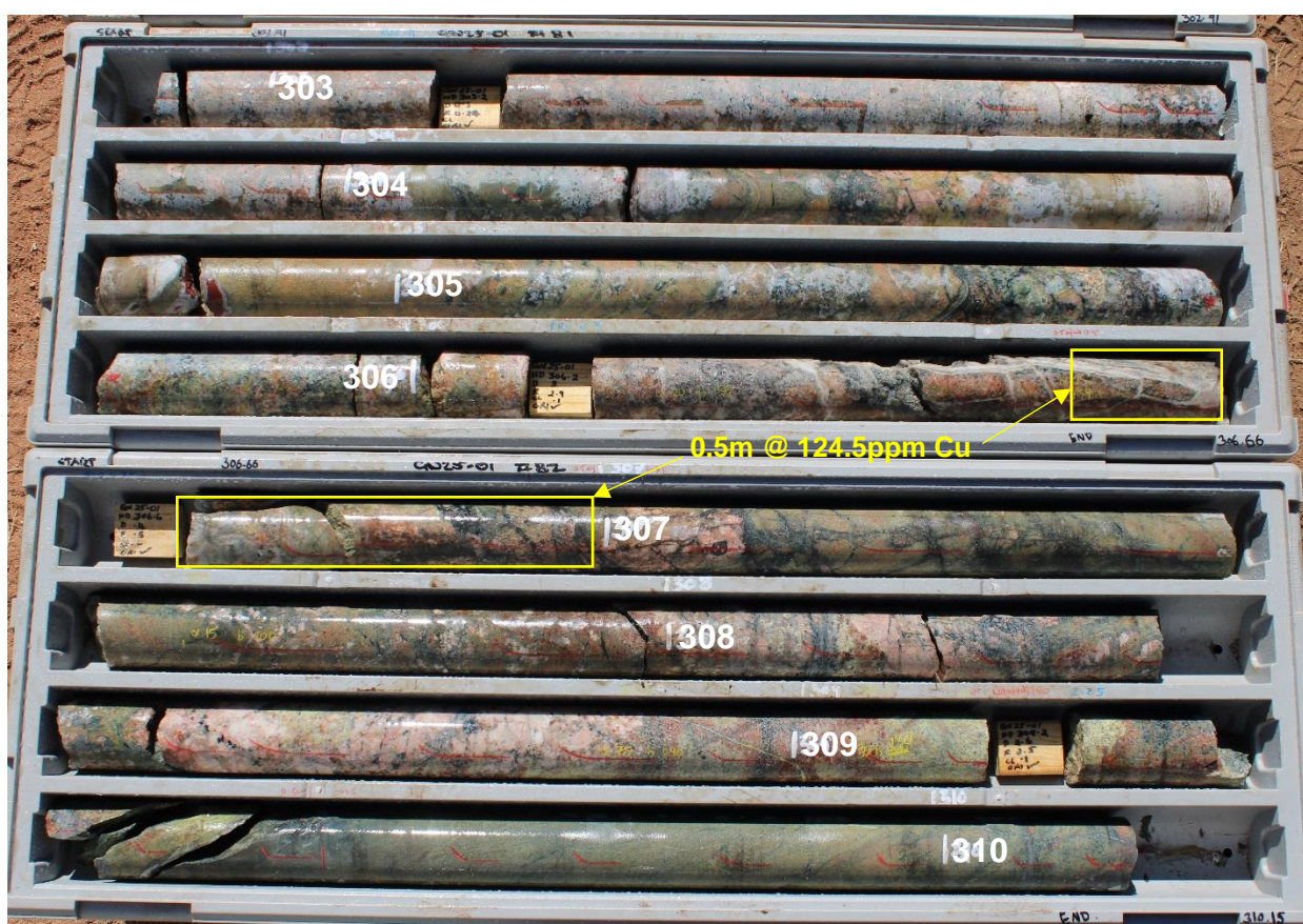
Figure 1 – Interval from GN25-01 showing elevated Cu associated with epithermal veining (incl. hematite and pyrite) in altered, brecciated granite
