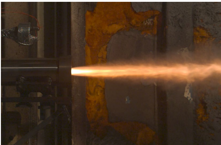
Figure 1A static test fire of an additively manufactured pressure vessel for a solid rocket motor. (Photo Credit: Northrop Grumman)
