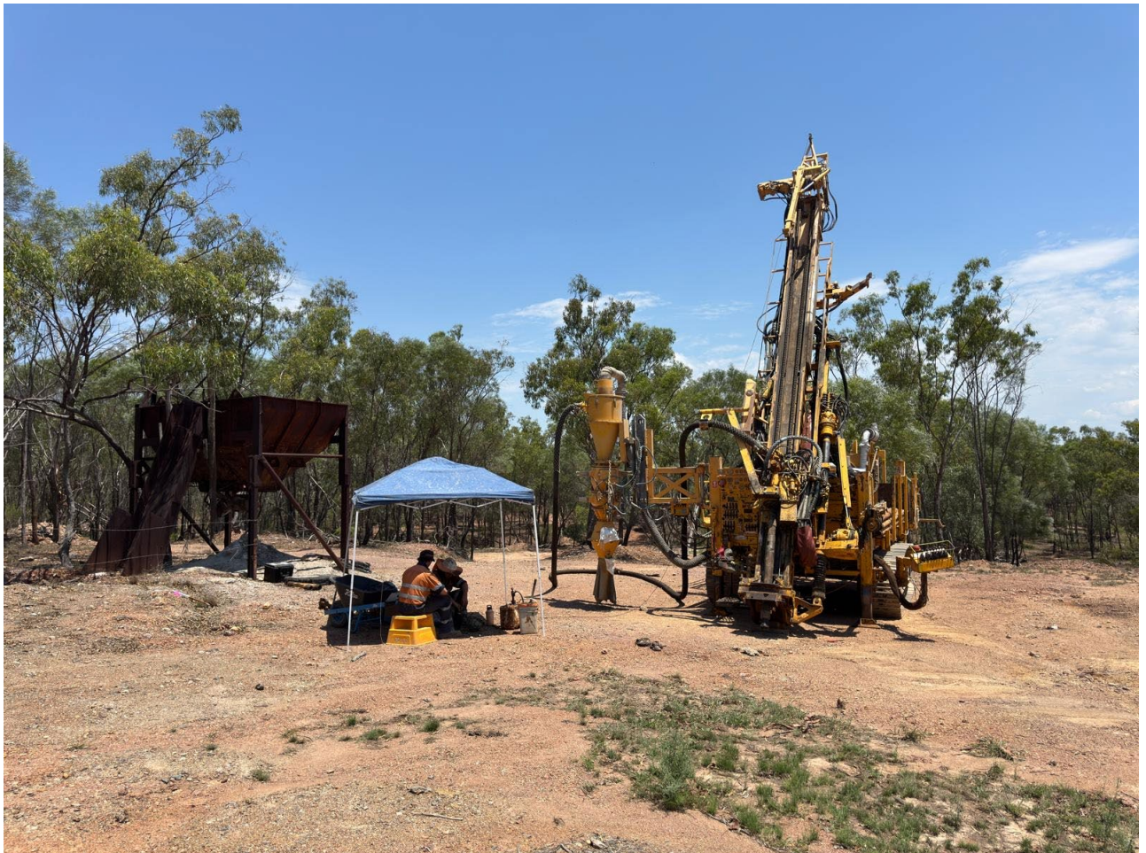
Figure 2: RC grade control rig setting up at Liontown.
