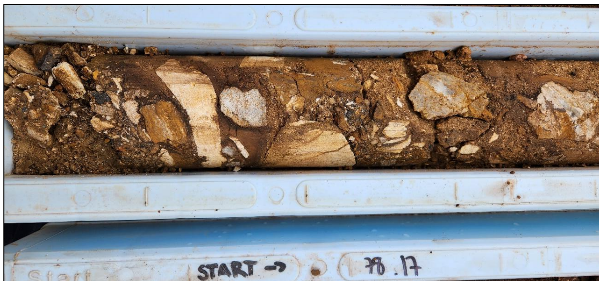
MLJDD020_178.0m_Polymictic Breccia with silica-pyrite clast
