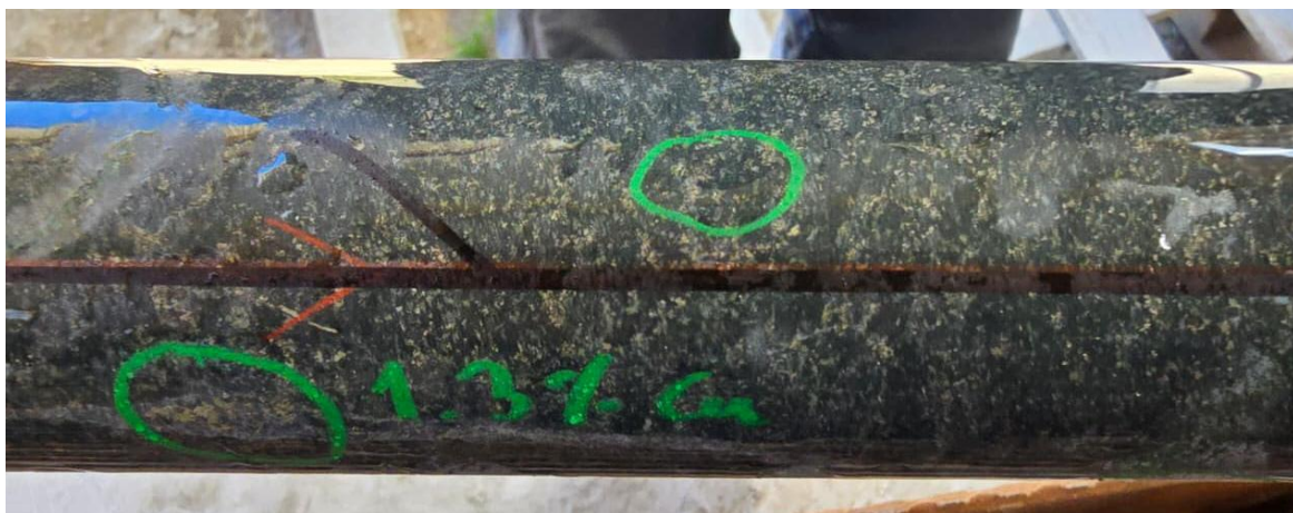
Photo 1. Disseminated sulphide mineralisation from a zone at 1268 to 1276.5m downhole in 25LHDD0070* (refer to Appendix 1).
