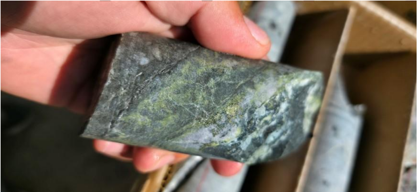
Photo 2. Anhydrite vein with chalcopyrite within altered porphyry from 1162.3m downhole* (refer to Appendix 1).
