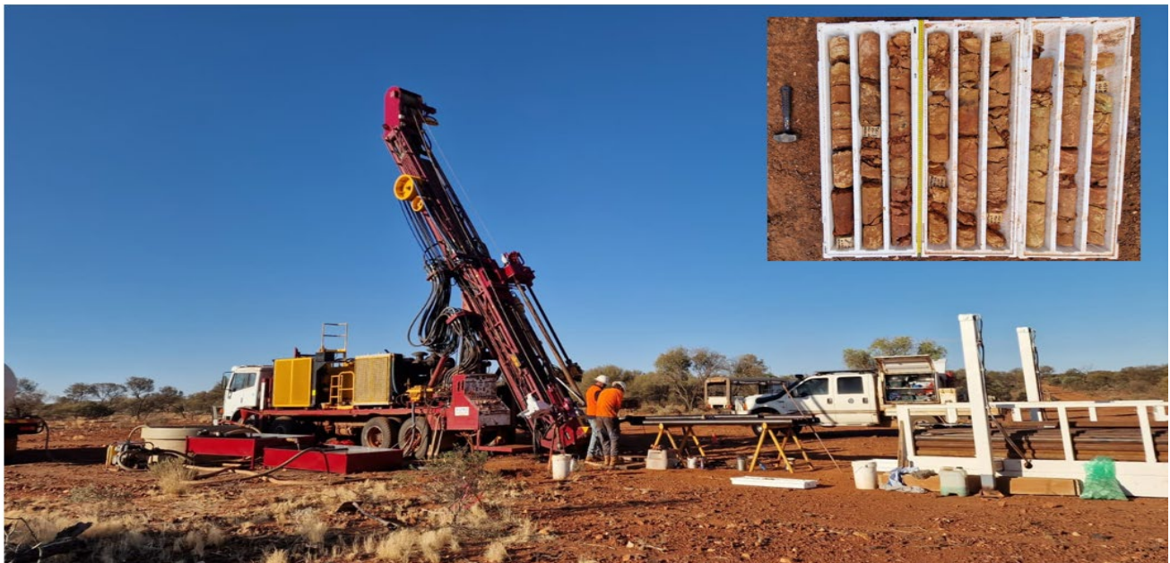
Figure 7 – Diamond rig drilling wide diameter core for heap leach amenability and gold recovery testwork on near surface low grade oxide and transition material. The inset image is an example of the wide-diameter core to be analysed.
