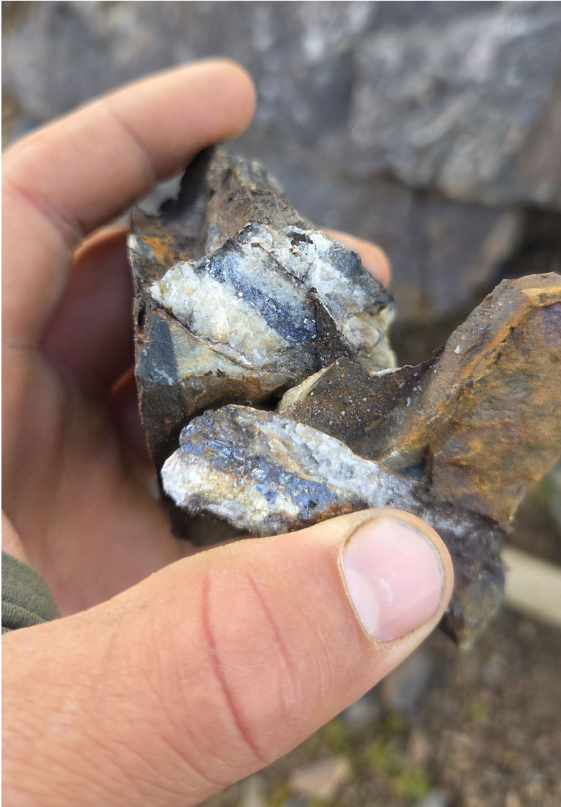
Figure 8: Field photo of rock float from 642885e 6986642n that is not in situ with 1-2cm quartz veins with visible arsenopyrite and stibnite mineralisation to demonstrate the style of veining present in the hornfels zone around the Tombstone stock (this rock float has not, and will not, be assayed).
