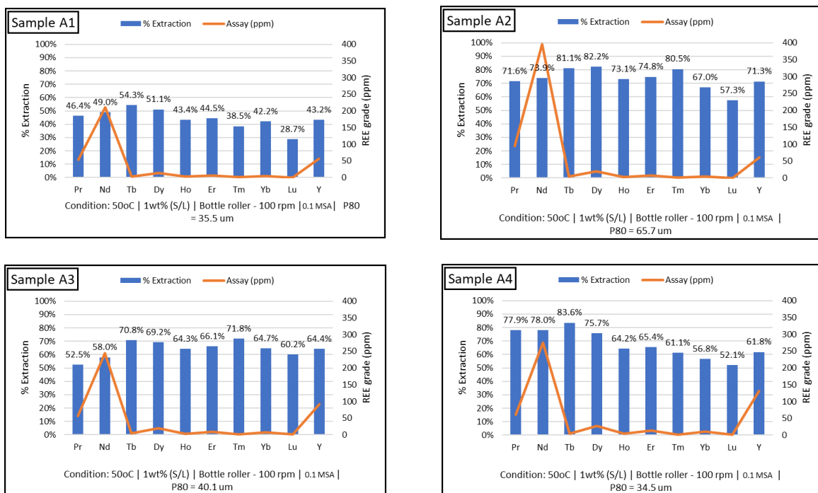
Figure 5. Extraction efficiency and grade of REE, across the 4 samples from Rocky Gully, applying MSA acid digest
