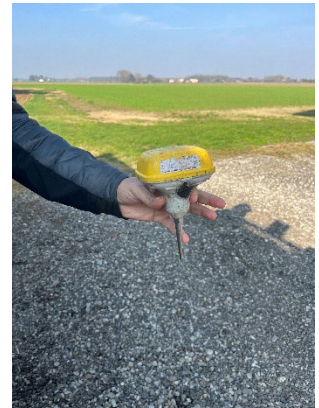
Image 6 – Wireless receiver node
