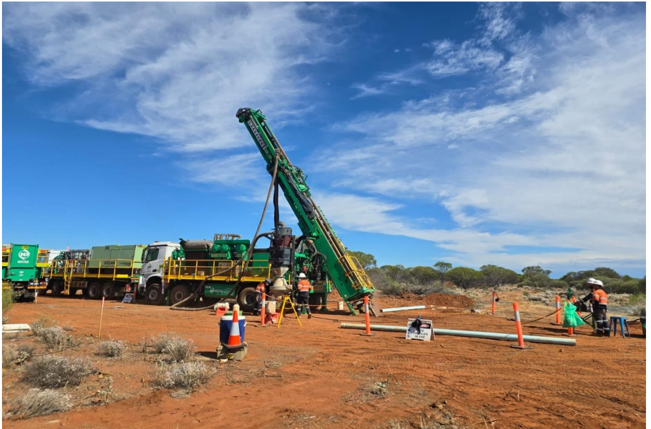
Figure 1: RC drill rig on site at Blue Heaven deposit (North pit) Murchison South Gold project
