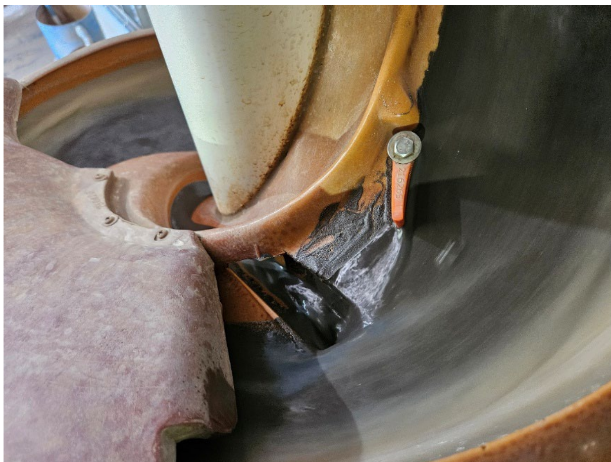
Photo 2: Rosewood HM sample being fed through a recleaner spiral at IHC Laboratories. Darker HM minerals on inner side of the spiral are split off as part of the HMC concentration process.
