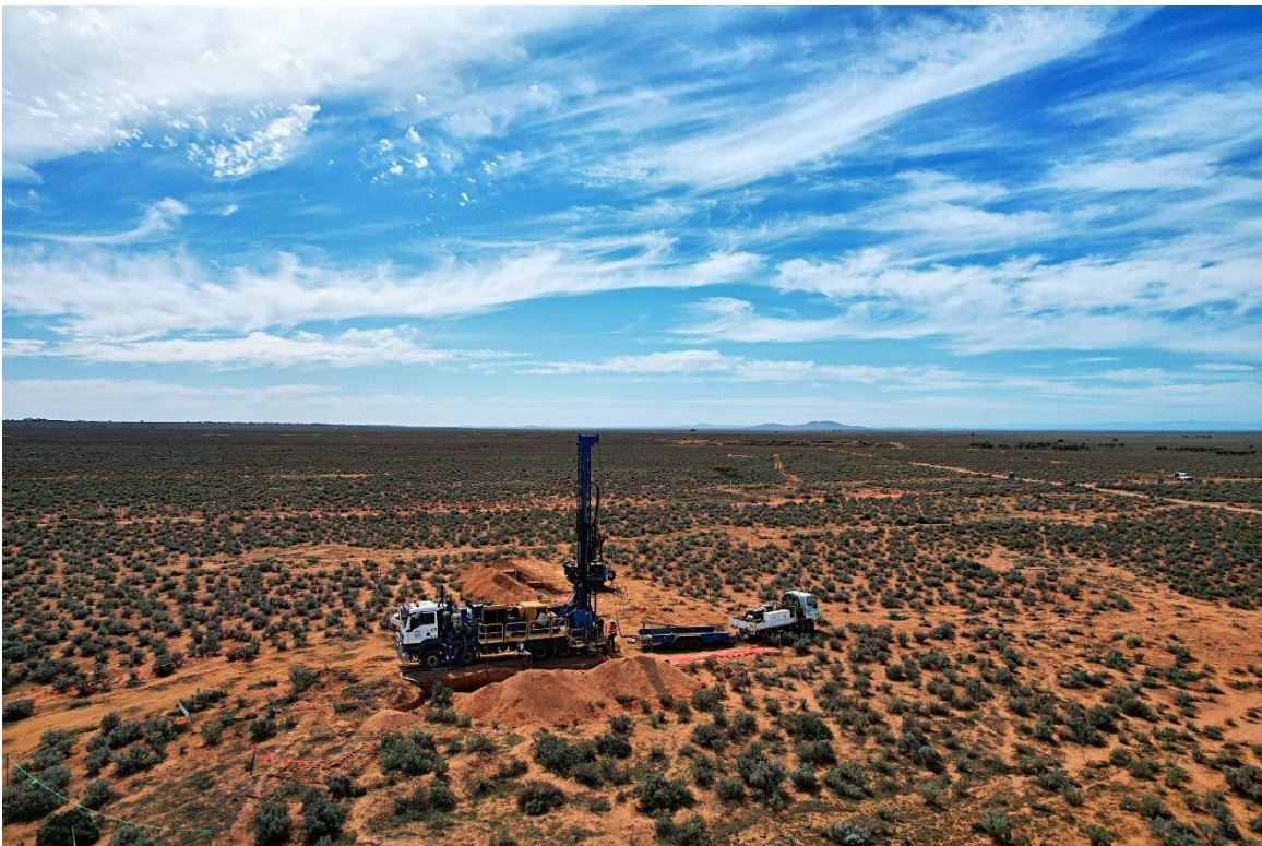
Figure 2 – Rig drilling an extractor as part of a recovery well pattern at Samphire.
