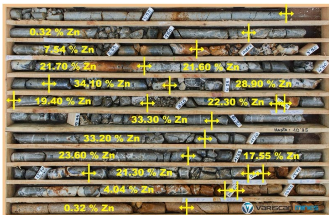
Figure 3: Diamond Drill Core from NDDT059 (15.3m @ 17.42% Zn, 4.40%) illustrating massive sphalerite hosted in dolostone. Hole depth shown is from 0.00m to 16.95m
