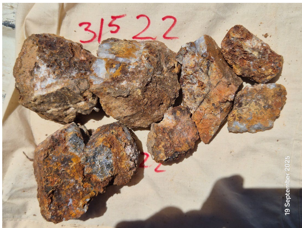
PLATE 2: Sample 13522 from trench QWTR02 at the Queenslander Workings (See plate 1). Channel sample across 1m wide zone of quartz veining and stockworking in granite. Limonite stained vughs after sulphides. Gold assay 25.5 g/t.
