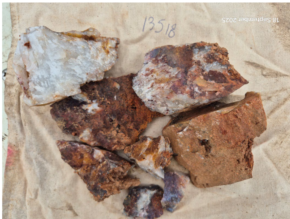
PLATE 5: Sample 13518 from trench GNTR03 at the Goldsmith North Workings (1.48 g/t gold). Channel sample of 50cm wide massive buck quartz with iron staining. Sheared and recrystallized quartz with limonite stained vughs.
