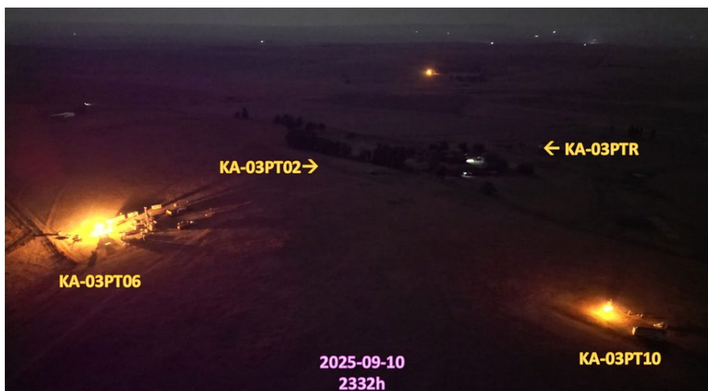
Figure 3: Production Test Well KA-03PT06 being choke tested with ongoing flow testing at well KA-03PT10 (the two other wells are shut in)
