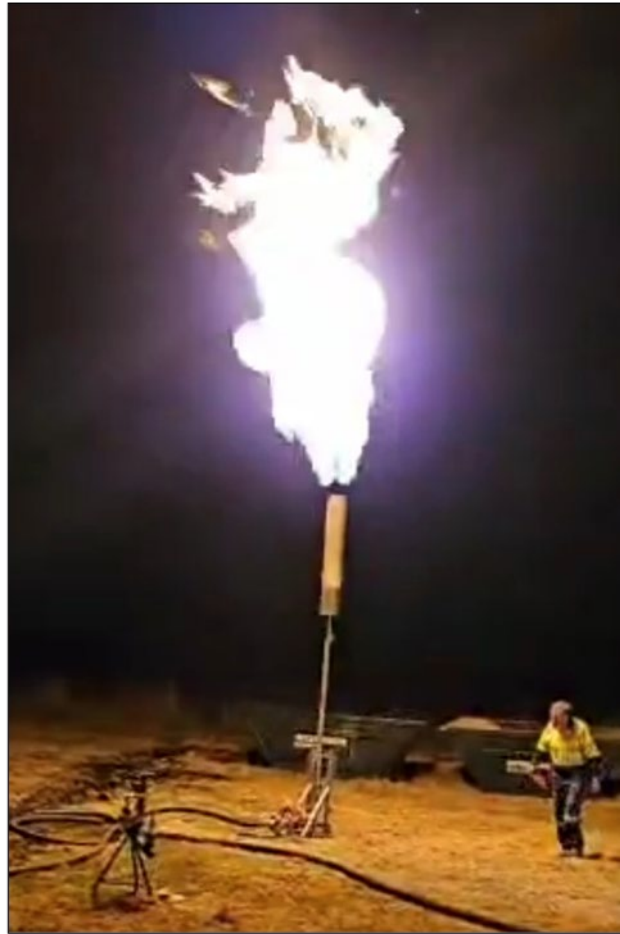
Figure 2: Production Test Well 271-KA03PT06 being choke tested
