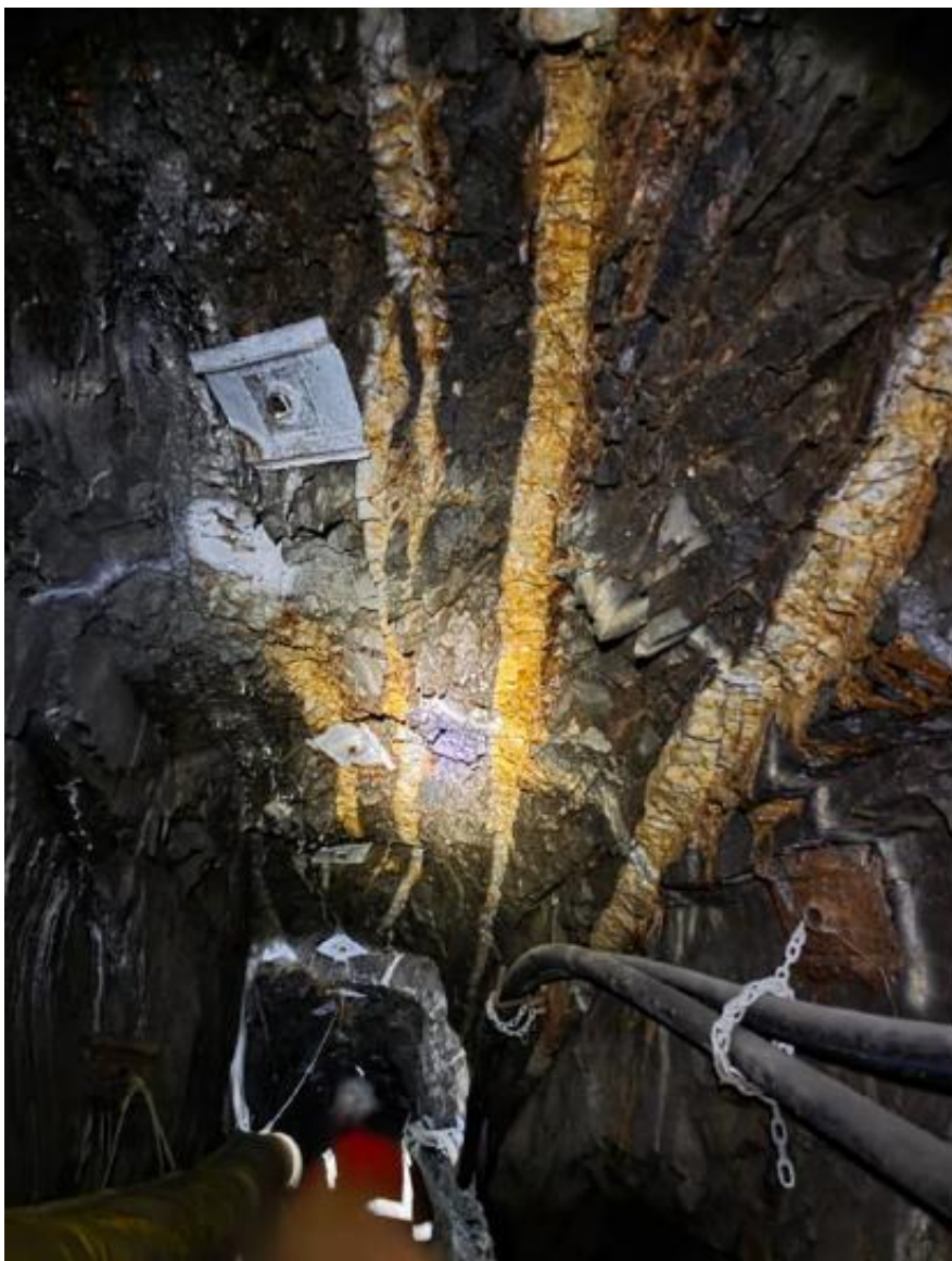
Image 6: High grade veins in the back of the 1670 Shrink Stope
