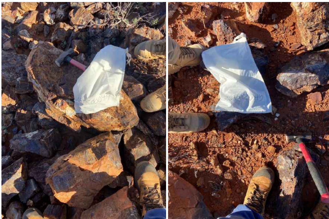
Figure 07: Mineralised samples (MGTS00044 and 45) of fractured, quartz-veined BIF.
