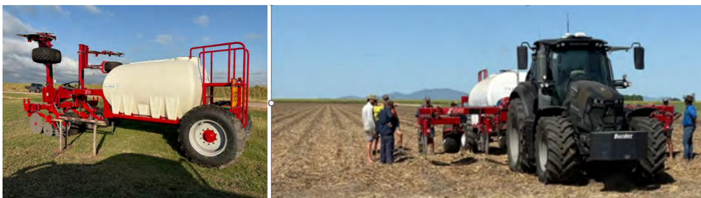
Figure 3: RLF Liquaforce variable-rate liquid applicator ready for first use in Ayr, Queensland (left). North Queensland growers discussing the applicator's first run (right).
