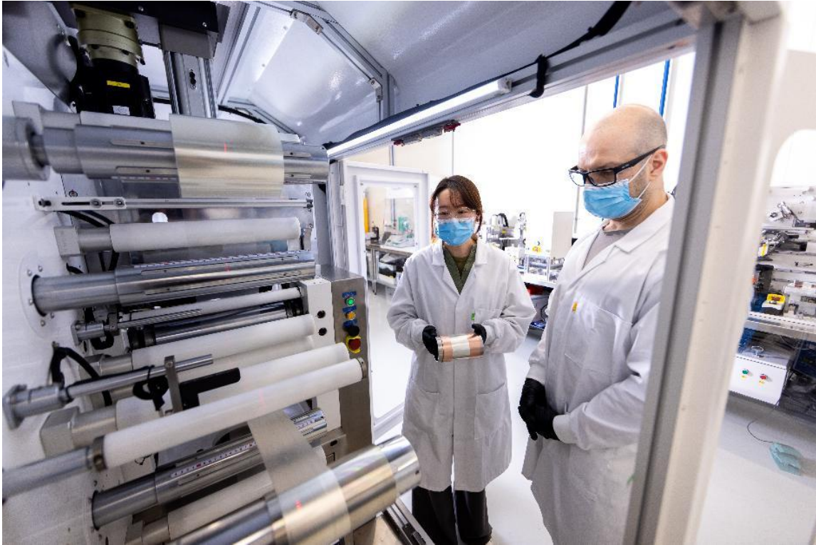
Image: Li-S Energy staff monitoring the laminating process housed inside the Li-S Energy production dry room
