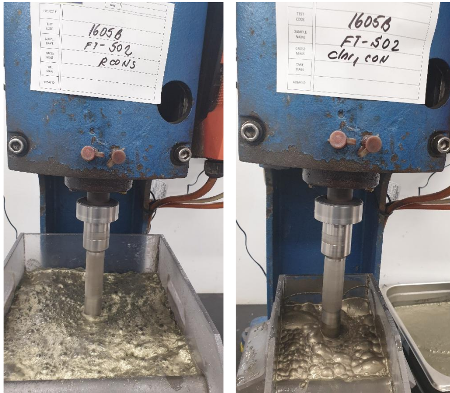
Figure 16: Copper concentrate from Kabikupa fresh composite – chalcopyrite is the major copper mineral
