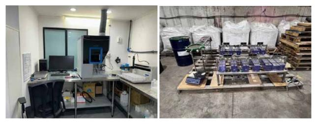
Figure 1.12. (L). ICP analytical machine capable of reading up to 66 elements to ppb levels of detection.
