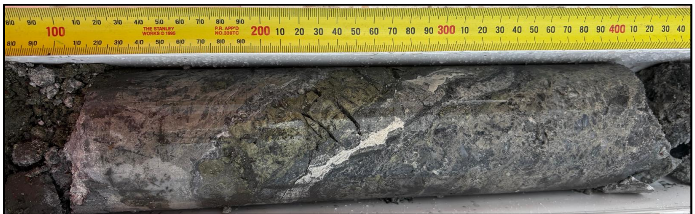
Figure 3 Semi-Massive chalcopyrite (25IRC011D) from 163.2-163.7m - assaying 4.59% Cu
