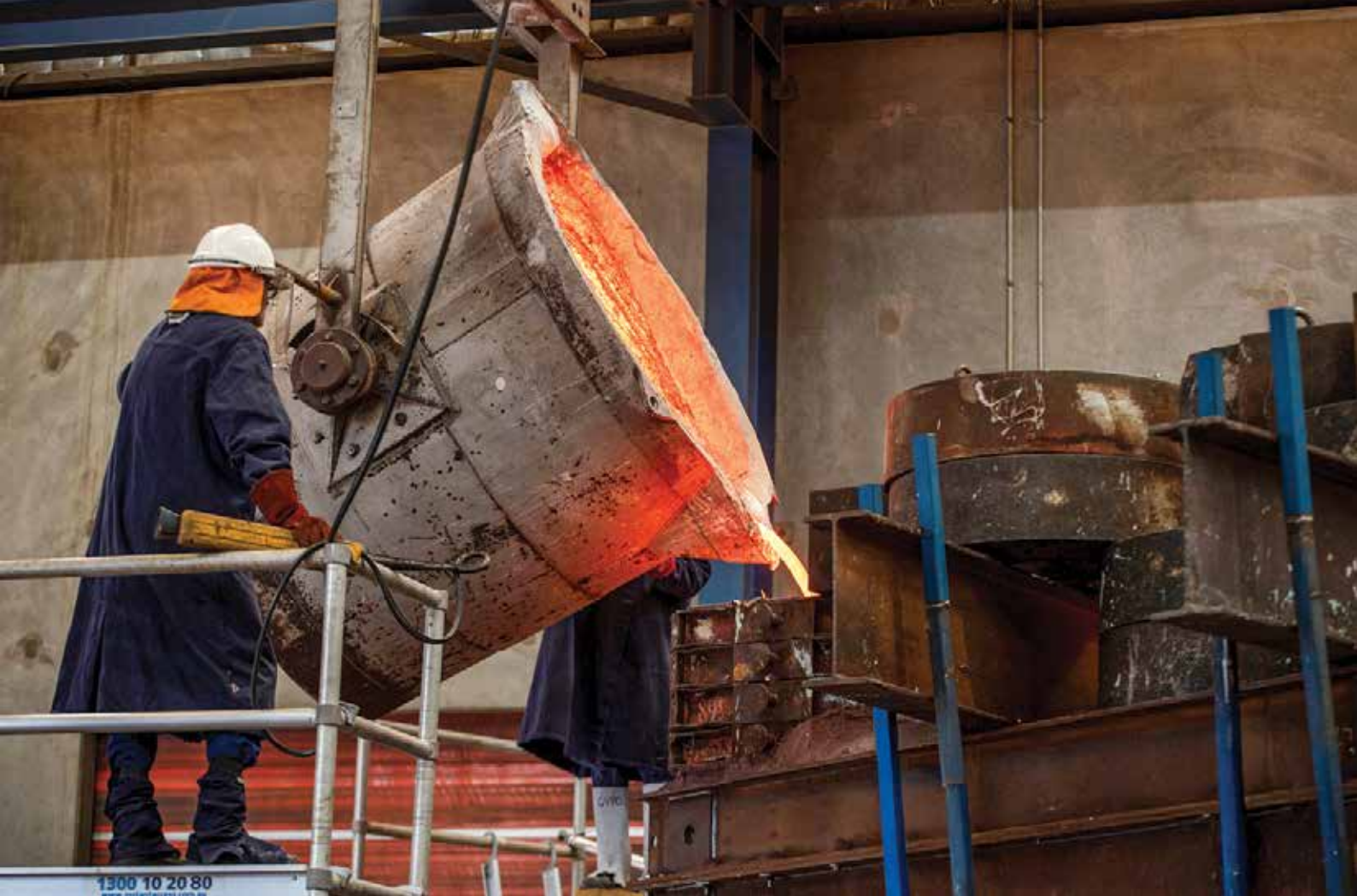
15.5 tonne casting being poured
