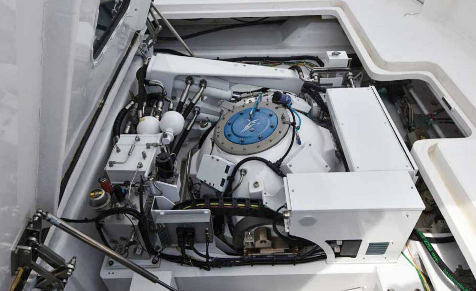
VG52 installed on the VEEM test vessel
