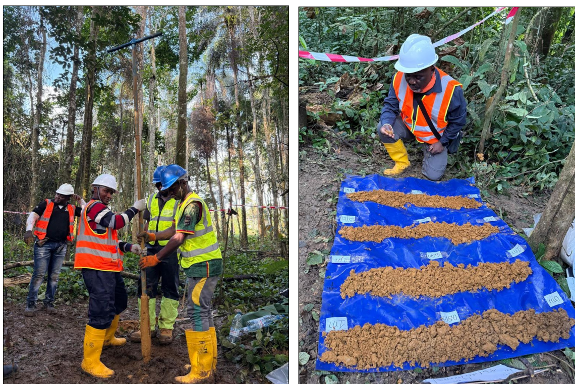
Figure 4 : Hand auger drilling team at the drill site LIPAU001 on the left and DY6 country manager Dr. Moses Ndasi inspecting the samples on the right.
