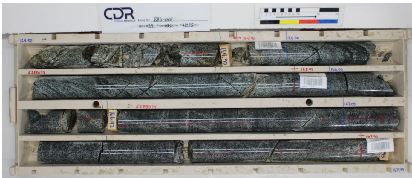
Figure 2. BRD001 altered granodiorite zone 10.3m from 155.6m at 0.55 g/t Au including 1m at 2.42 g/t Au m from 164.9m.
