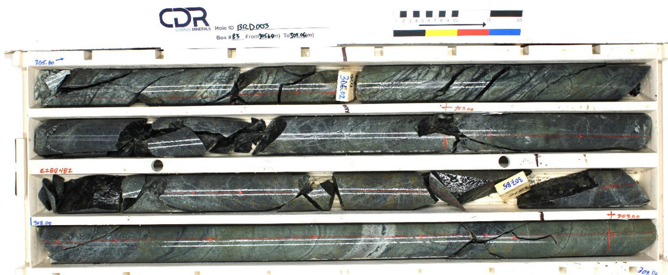
Figure 3. BRD003 strongly altered diorite including 4m from 305m at 1.52g/t Au.
