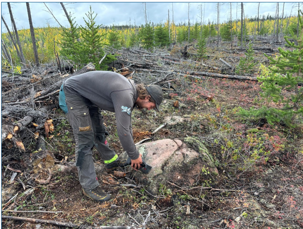
Figure 2: Field team on site at Reitenbach Lake mapping and using the RS-125 Scintillometer to gather and assess the radioactive readings, 59 locations were noted to record scintillometer readings exceeding 1,000 counts per second with a maximum of 9,700 counts per second 1 , indicating significant localized radioactivity.
