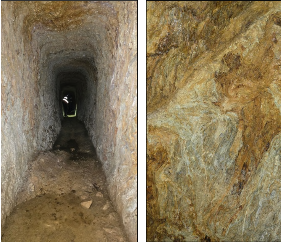
Figure 2: Previously undiscovered adit exposing a west dipping strong altered reverse fault zone (MGA94 Zone 55; 376,013mE; 5,333,824mN)
