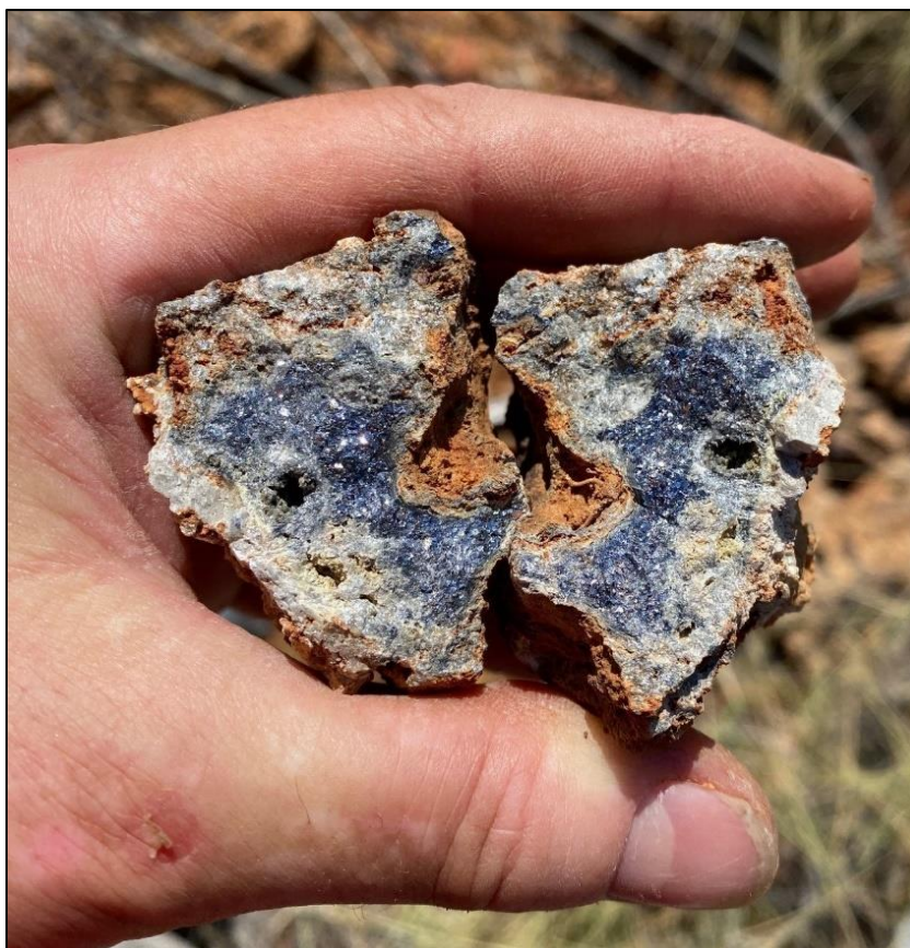
Figure 4. Sample RS0061024 from the Pickand's Showing displaying massive galena and iron oxide staining in silicified mafic volcanic.
