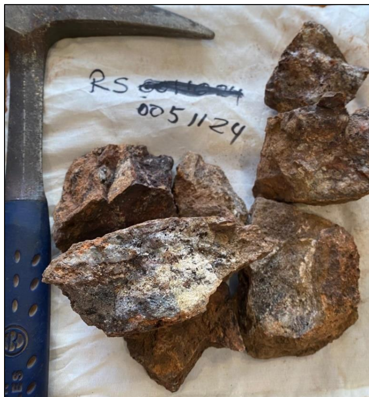
Figure 5. Sample R0051124 from Appaloosa showing iron oxide stained quartz veins in gabbro
