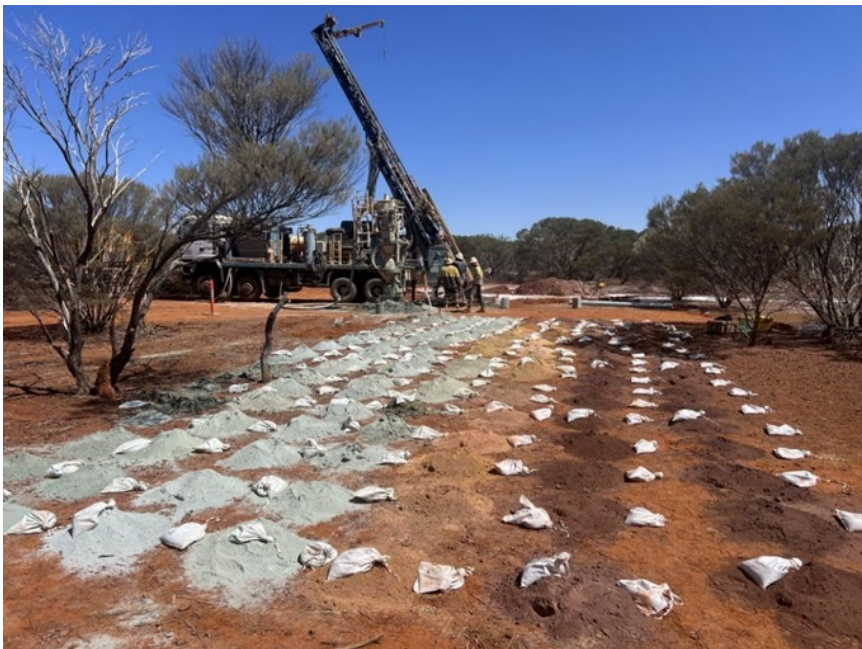
Plate 1. Challenge Drilling – Drill Hole VCR012- Vulcan with 1 metre samples
