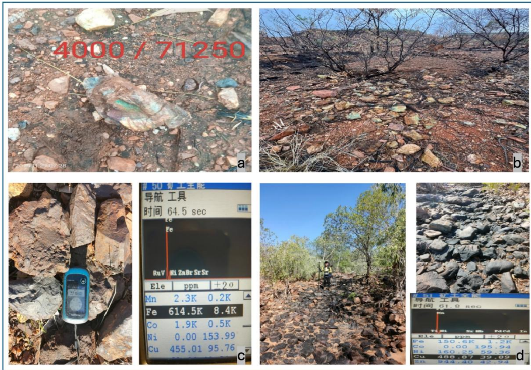
Figure 4: Photos illustrating high grade oxidized copper ore, mainly malachite (a, b), magnetite quartzite (c) and meta-mafic unit). Note that P-XRF analyses reading are indicative only for guiding further test work. *Visual estimates of mineral abundance should never be considered a proxy or substitute for laboratory analyses where concentrations or grades are the factor of principal economic interest. Visual estimates also potentially provide no information regarding impurities or deleterious physical properties relevant to valuations.
