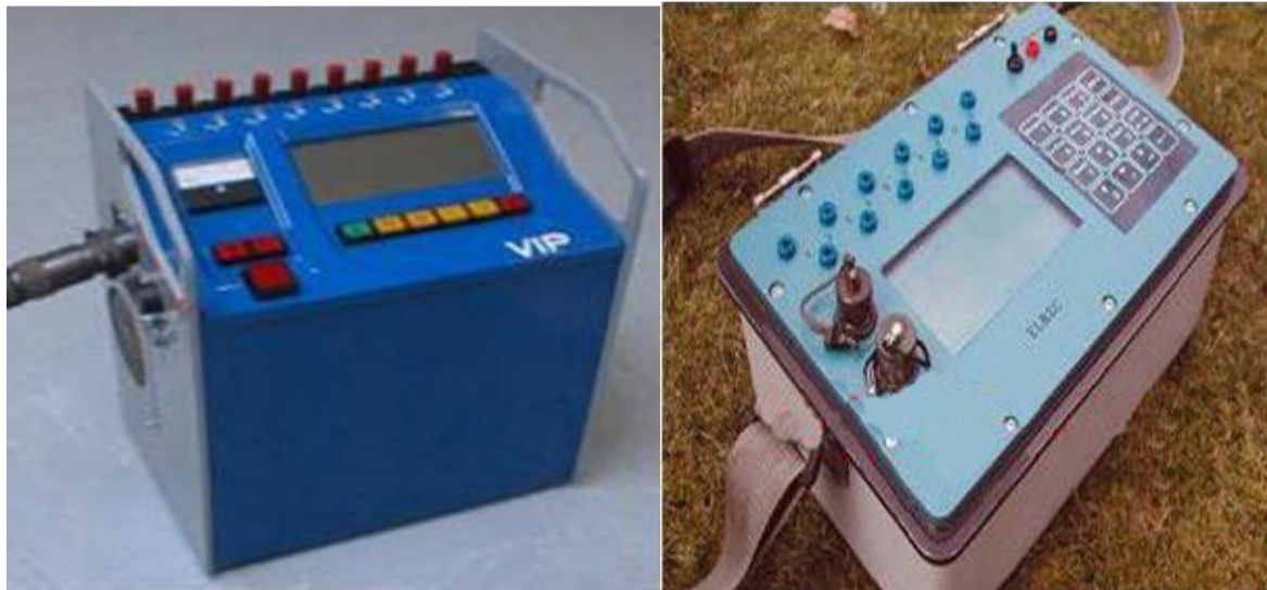
Figure 7: VIP 5000 I.P. transmitter and receiver
