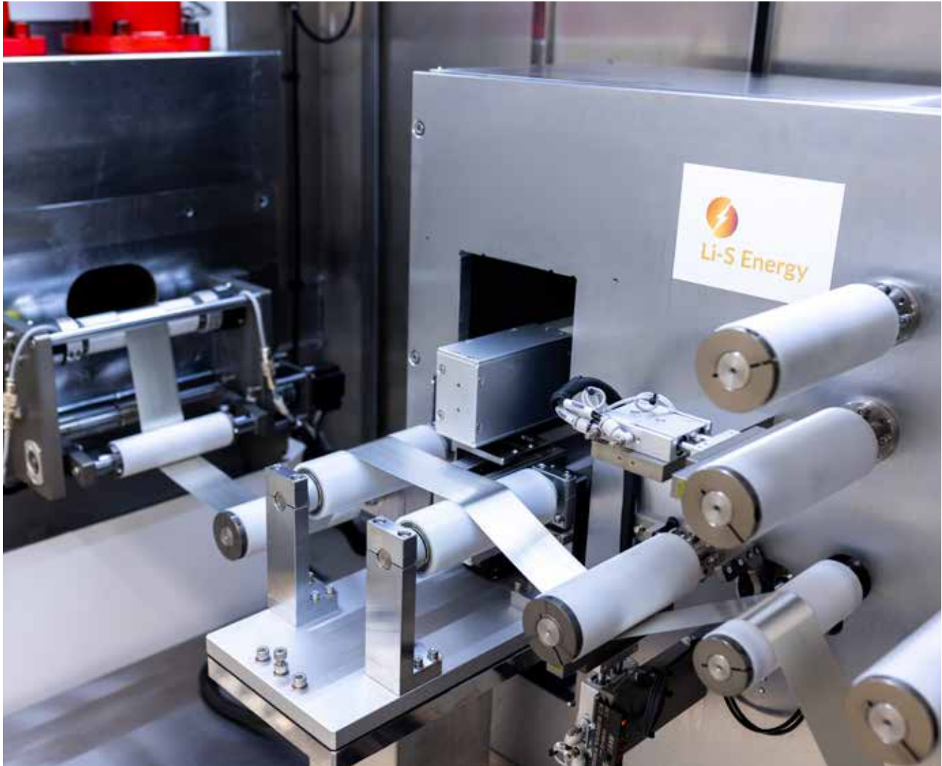
Li-S Energy's Lithium Extruder manufacturing ultra-thin lithium foil
