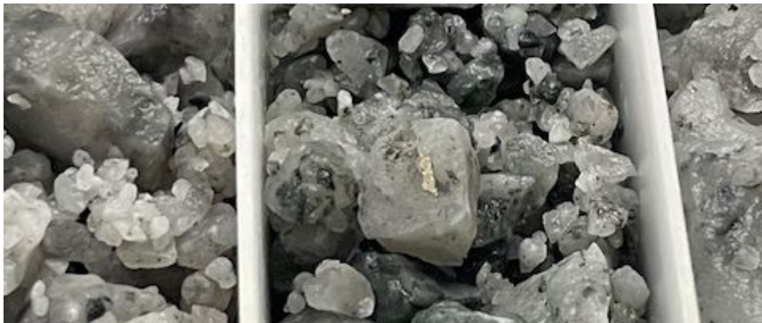
Plate 1: YBRC 137 Prominent blebby Sulphide ( pyrite/arsenopyrite/chalcopyrite ) in quartz zone at 172m. Relative abundance of sulphides estimated to be 2-4% 1
